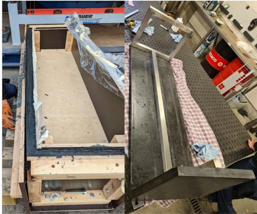
Figure 4. First Bench. Left: Demoulding, Right: Addition of steel frame to bench for supporting the broken leg.
